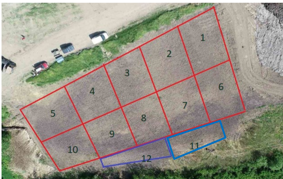
Figure 5-6. Division of Landfill 1 into control (11,12) and experimental (1-10) sections
