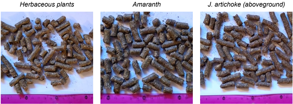
Figure 6-8. Pellets of the biomass obtained at Lithuania pilot site field trials in 2022
