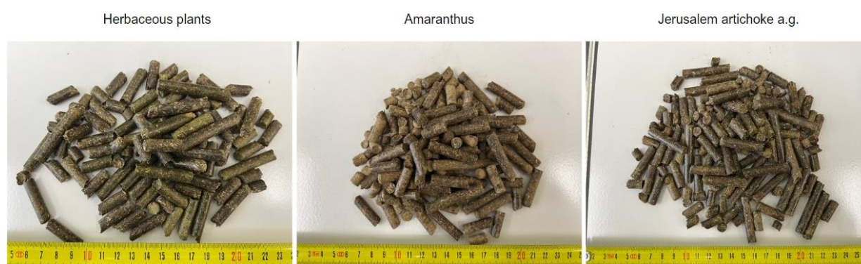
Figure 6.8. Pellets of the biomass obtained at Lithuania pilot site field trials in 2023
