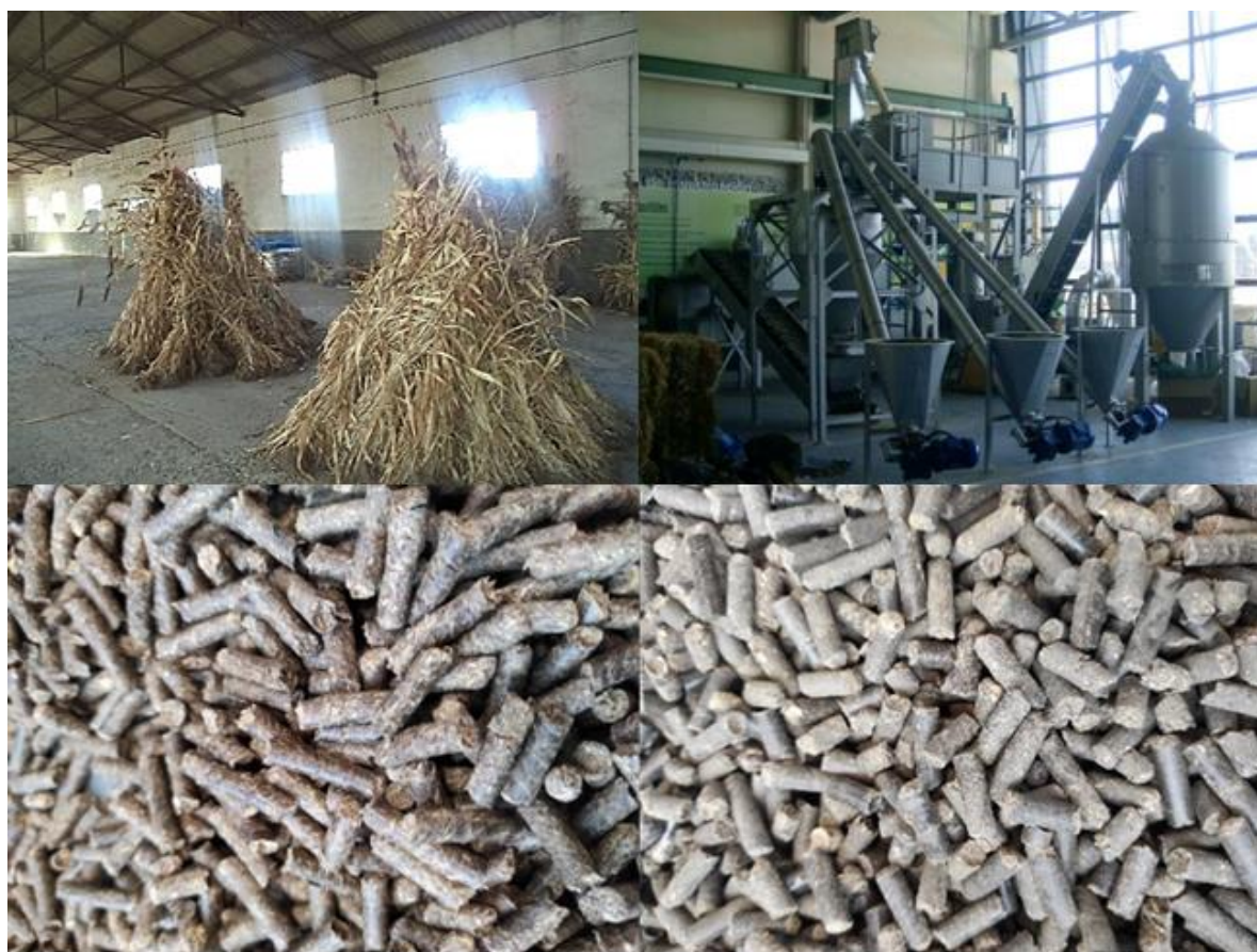
Figure 4.10. Drying process of biomass (upper left). Biomass treatment and pelletization plant (upper right). Sorghum biomass (2022) pellets obtained with a compression ratio of 1:4 (lower left). Sorghum biomass (2022) pellets obtained with a compression ratio of 1:6 (lower right).
